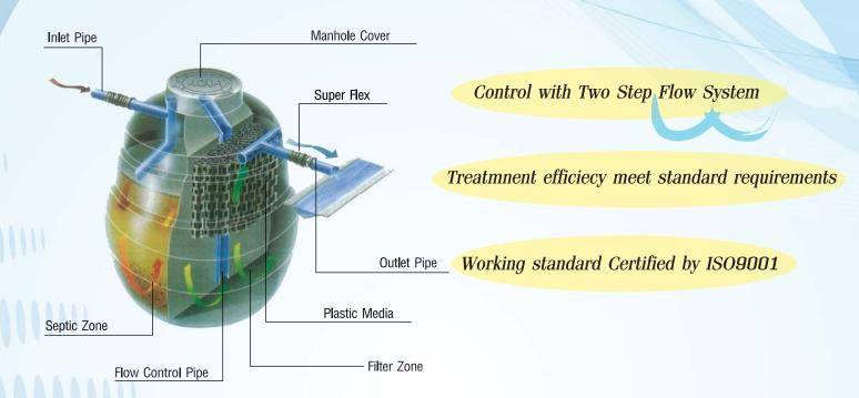
**AQUA PAC** is a package treatment tank. AQUA PAC consists of septic and anaerobic filter chamber in one tank. It is suitable for wastewater from residential area to small offices. Treated water will have quality meeting the effluent standard and can be discharged without adverse effects to environment.
