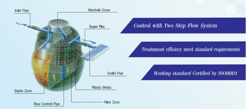
**AQUA PAC** is a package treatment tank. AQUA PAC consists of septic and anaerobic filter chamber in one tank. It is suitable for wastewater from residential area to small offices. Treated water will have quality meeting the effluent standard and can be discharged without adverse effects to environment.
